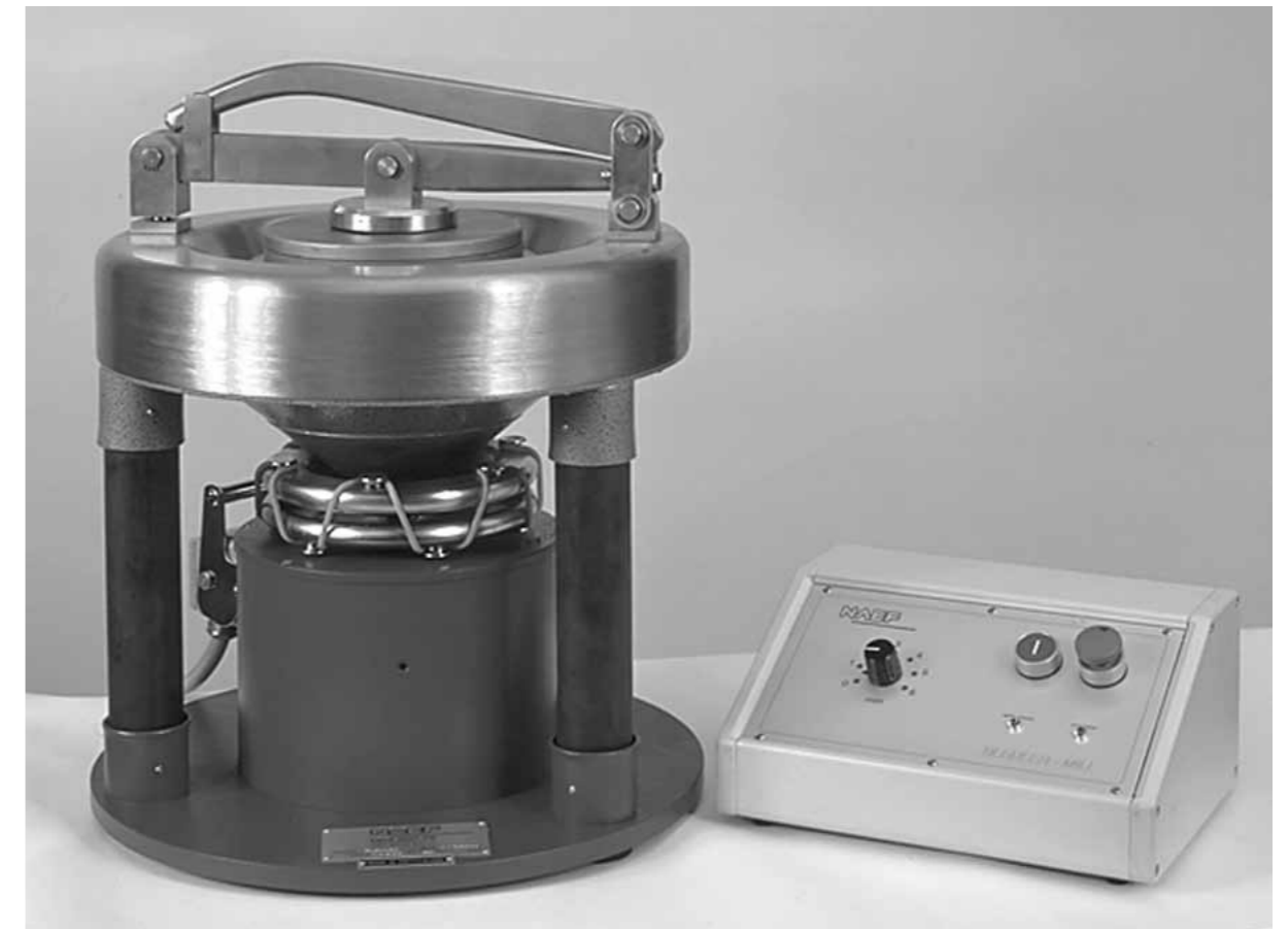
Mill and Control unit
